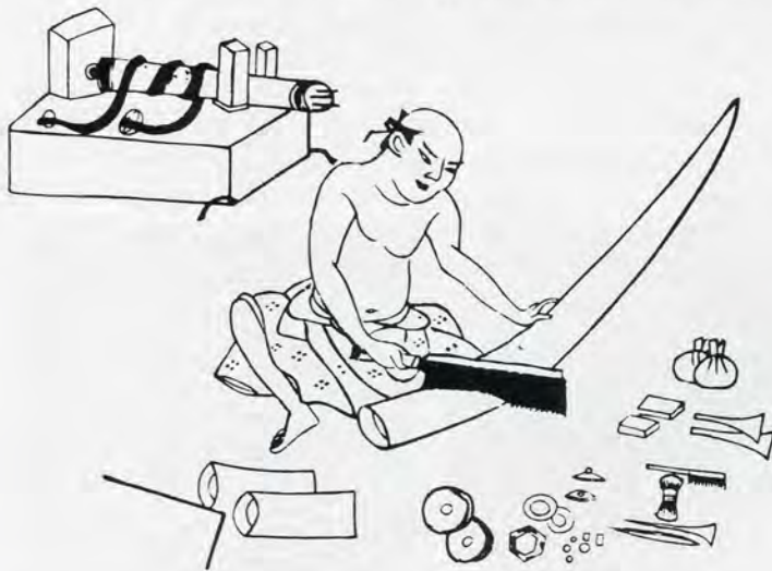
Fig. 4. Early ivory (or "horn") worker from 1690 book. Note use of whole tusk, cylindrical sections, multiple various "wares" and lathe in background.
